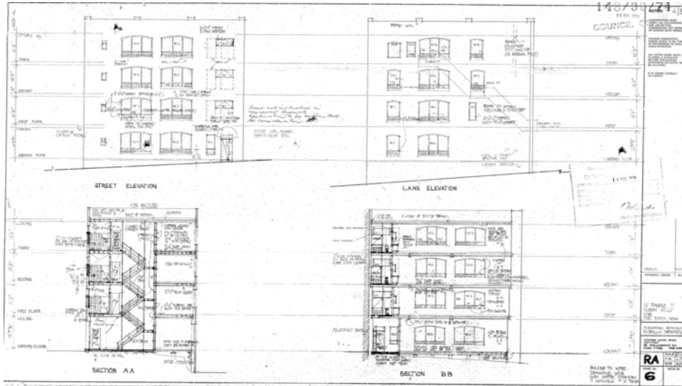
Figure 5.4.3A The building was badly damaged by fire in 1973 and was remediated the following year. That work was extensive. Elevations and sections by Stephen Javor. RAIA
