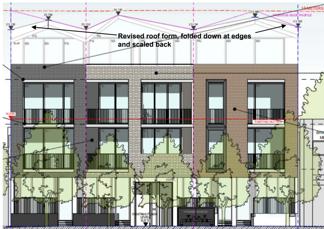
Figure 7: Revised Mitchell Road elevation, including a new masonry brick facade and a scaled back roof form.
