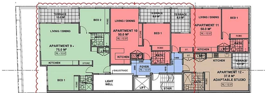
Figure 13: Third floor plan (final amendment).
