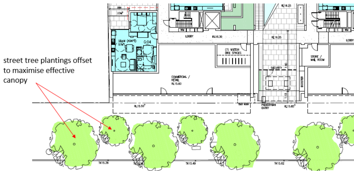
Figure 5: extract from submitted plan DA04 showing 'offset' planting to maximise canopy spread
