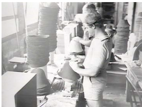
Figure 5.3.4 The second stage in the sanding of felt hat to remove any irregularity or blemish. March 1949
