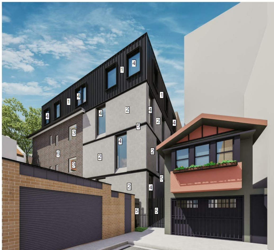
STANDING SEAM CLADDING - MONUMENT MATT (NON- COMBUSTIBLE TO AS 1530.1)
