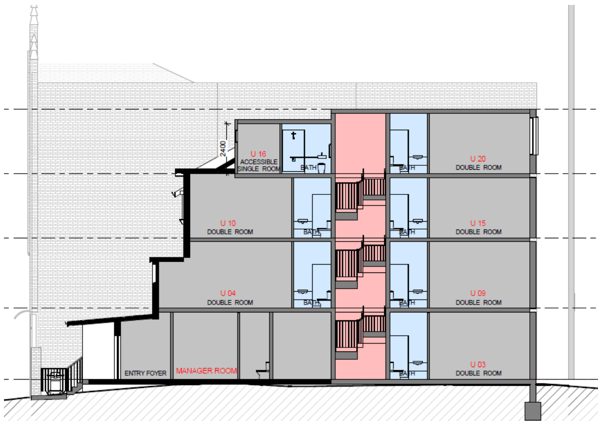
Figure 17: Proposed Side Section
