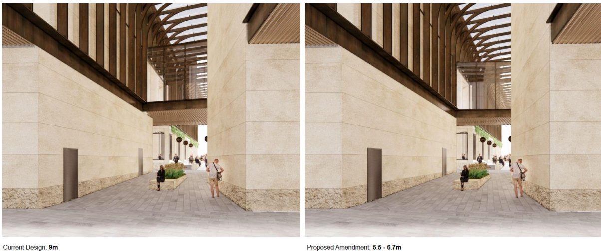
Figure 49: Original (captioned as Current) and reduced width (captioned as Proposed) bridge link over Queens Court as viewed from Underwood Street
