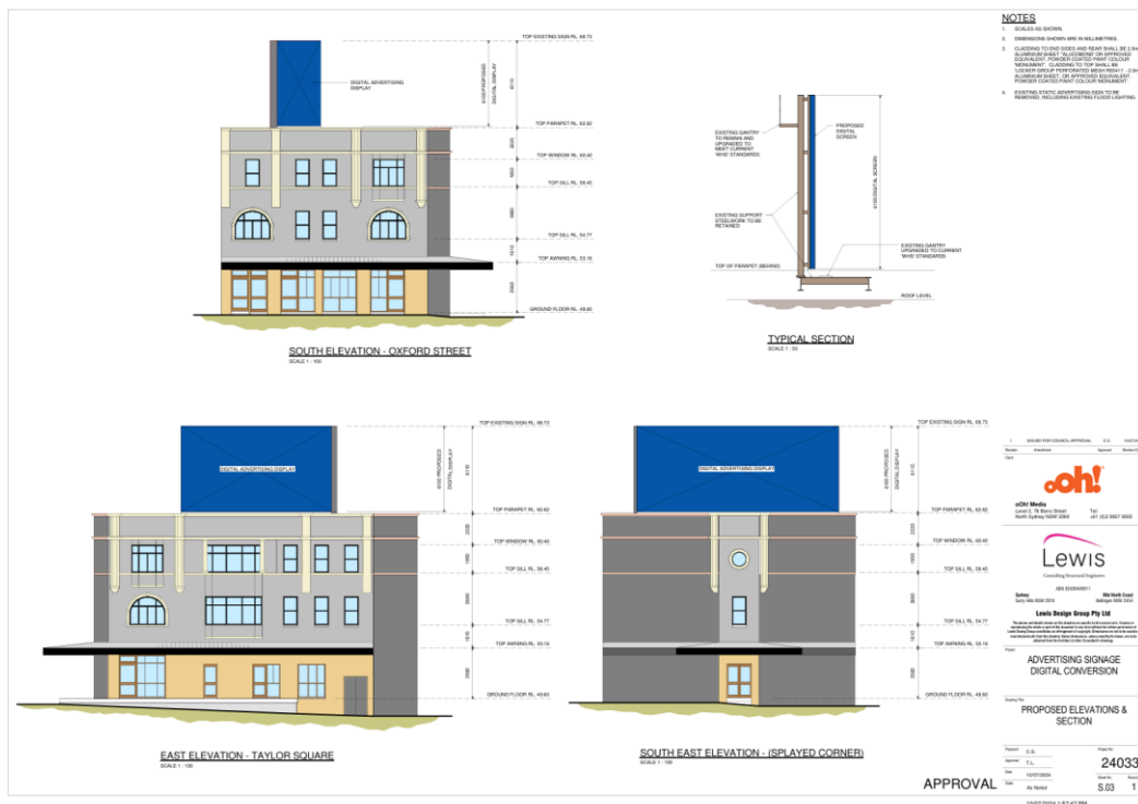
Figure 8 – Proposed Plan Elevations and Section (Source: oOh!Media)
