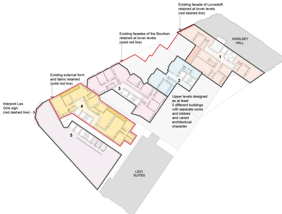
Figure 12: Concept typical upper level plan (of a predominantly residential level) showing how fine urban grain, retention of heritage fabric and variety of architectural characters can be achieved [figure 12 for information only – to be removed post-exhibition]
