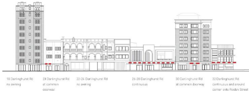
Figure 10: Elevation of the development block showing sections of street façade where entry awnings or interpretations thereof are appropriate (red dotted line)
