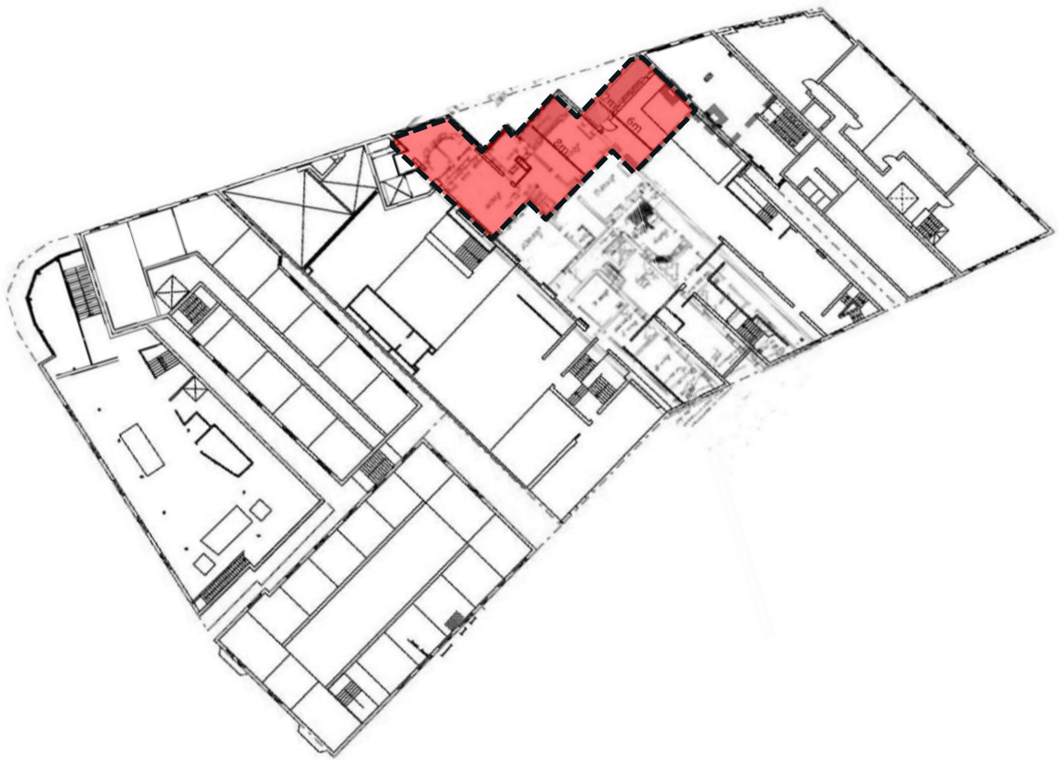
Figure 4a: Ground level plan of the Bourbon showing the extent of existing facade and internal fabric to floors and walls to be retained in dotted black outline, shaded in red
