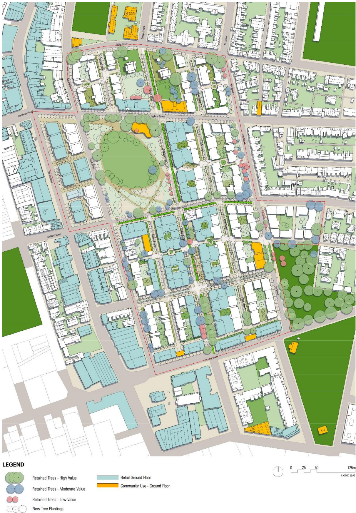
Fig 14. CoS alternate approach ground plane showing location of retail, services, and community uses.
