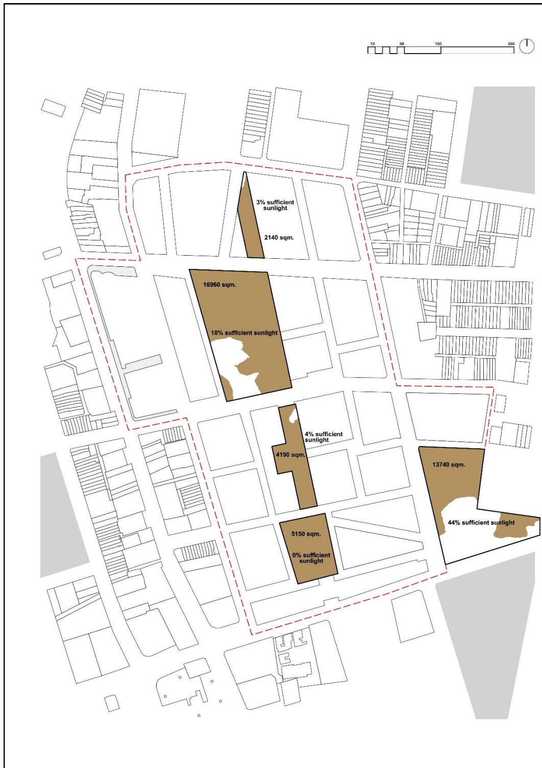
Fig 3. LAHC preferred masterplan showing the proposed two parks area of minimum solar access in midwinter (CoS modelling) and the residual solar access to Waterloo Park North (to the east of the Estate). Compare to Fig 2.
