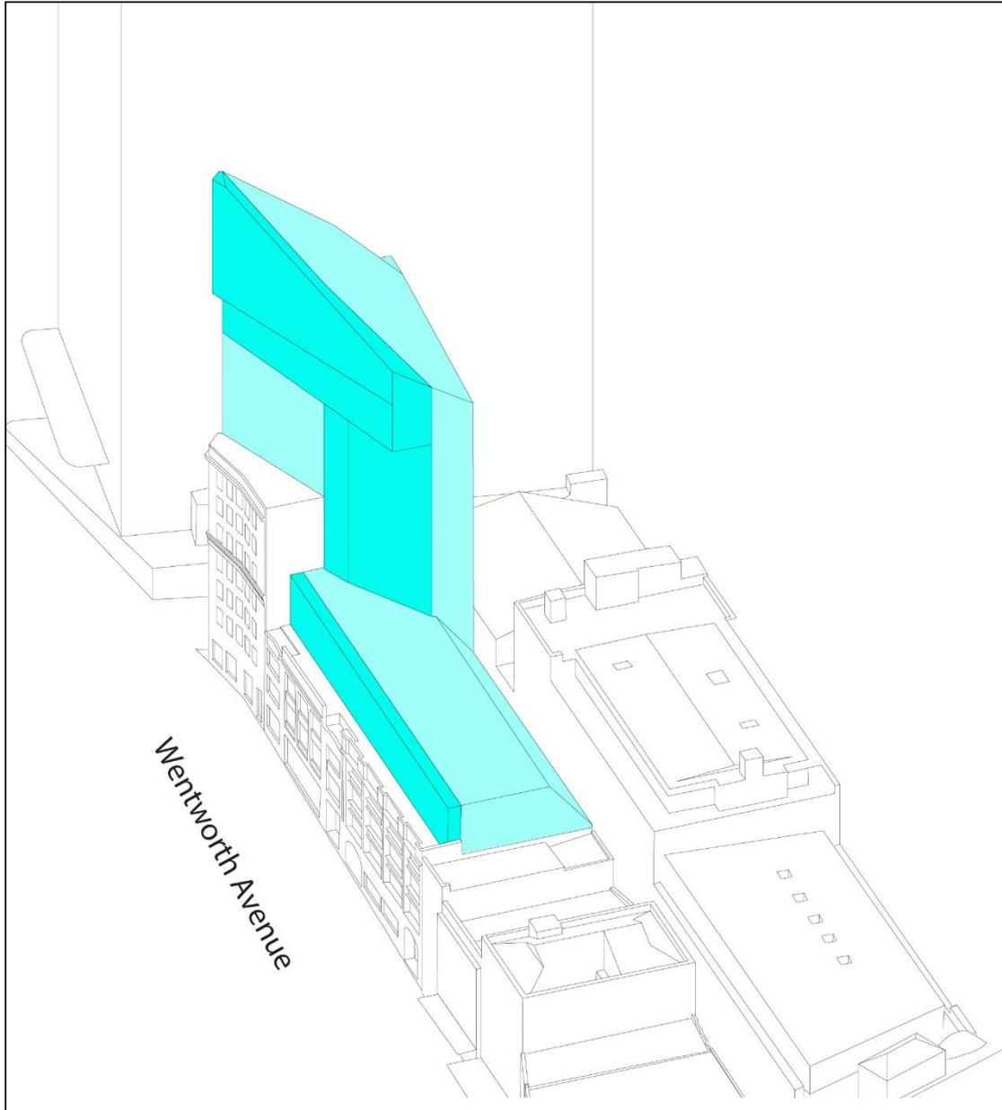
**Figure 6xxx: 4-22 Wentworth Avenue: Maximum planning envelope – axonometric view 1**
