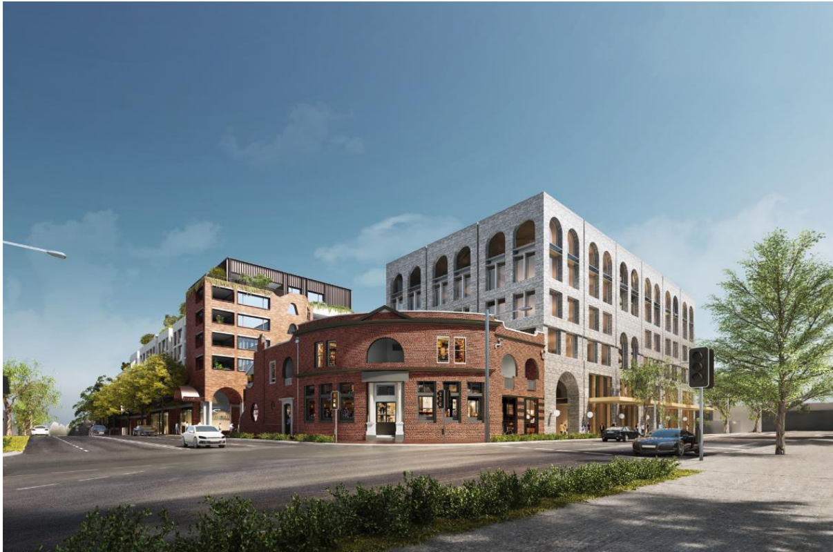
Figure 48: Proposed photomontage of Building G depicting the proposed CLT structure (internally) and the exterior brick cladding.
