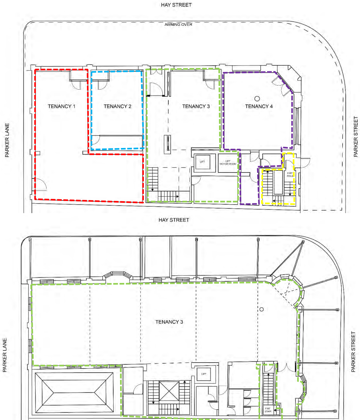
Figure 43 – Ground Floor (top) and First Floor (bottom) existing plans, with tenancies identified. Note: not all existing lightweight partitions in each tenancy identified.
