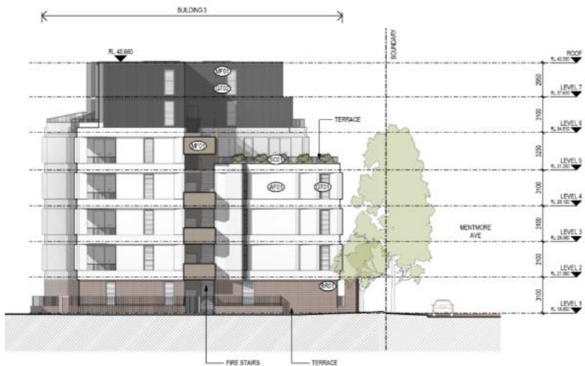
Figure 34: Proposed building 3 - south elevation
