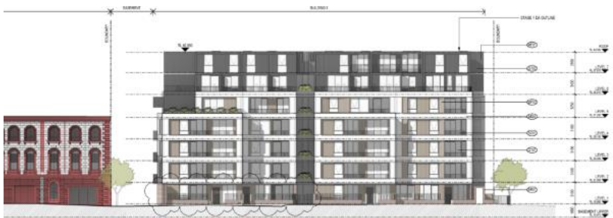
Figure 30: Proposed building 3 fronting Mentmore Avenue - east elevation
