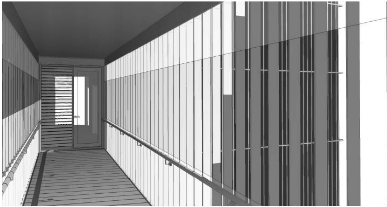
Figure 42 - Perspective of the breezeway with louvres and opening for light and ventilation
