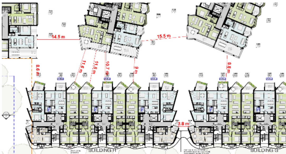
Figure 43: Level 4 plan marked up showing separation distances non-compliances. They should be separated by a minimum of 18metres.
