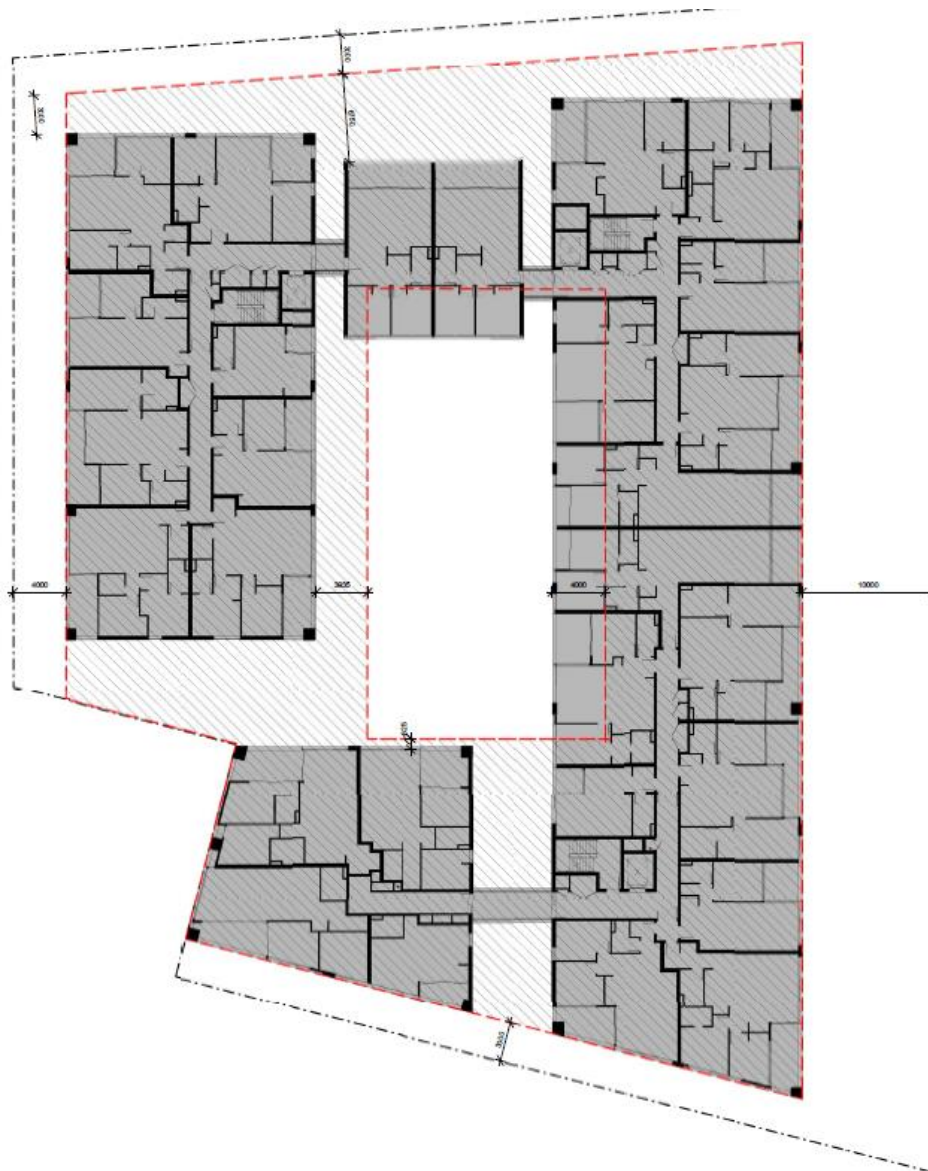
Figure 6 - Proposed building footprint in grey as shown in relation to the approved building envelope (hatched)
