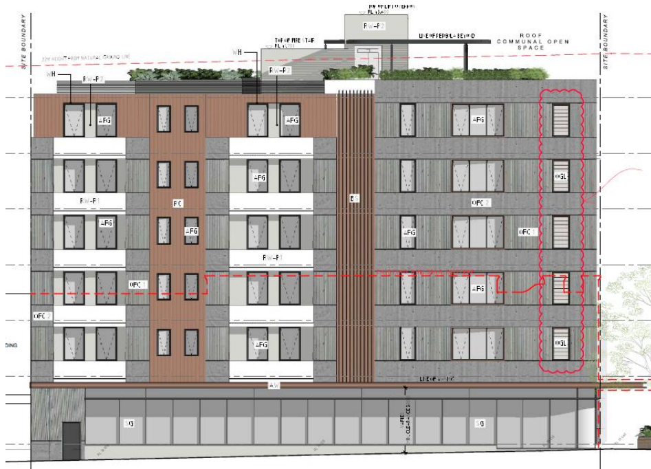
Figure 16: South elevation (Parramatta Road)
