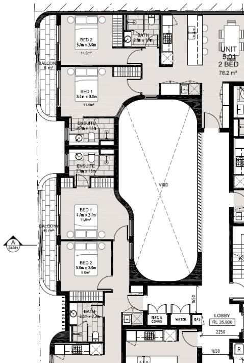
Figure 32: originally proposed floor plan, illustrating bedrooms with sole reliance on balconies to Parramatta Road
