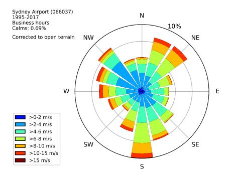
Figure 24 Wind rose showing probability of time of wind direction and speed
