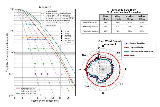
Figure 11: Probabilistic comparison between wind criteria based on mean wind speed (for the hours of 6 am and 10 pm) – Location 5
