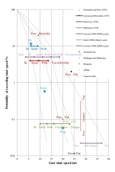
Figure 35 Probabilistic comparison between wind criteria based on 3 s gust wind speed
