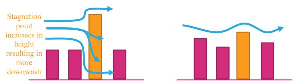
Figure 30 Schematic of flow pattern interference from surrounding buildings
