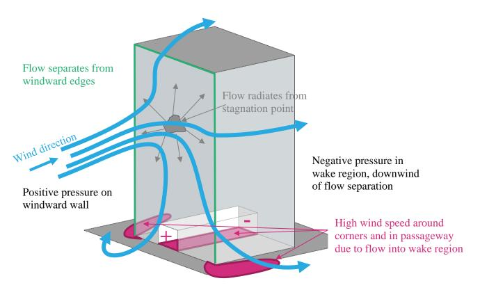
Figure 25 Schematic wind flow around tall isolated building
