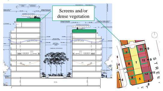
Figure 18: Recommended indicative rooftop terraces screens/dense vegetation in green: section (L) and plan (right)
