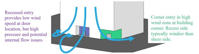
Figure 29 Schematic of flow patterns around isolated building with ground articulation
