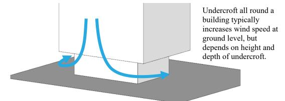
Figure 28 Schematic of flow patterns around isolated building with undercroft
