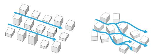
Figure 31 Schematic of flow patterns through a grid and random street layout
