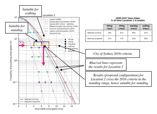
Figure 5: Probabilistic comparison between wind criteria based on mean wind speed (for the hours of 6 am and 10 pm) – Location 2
