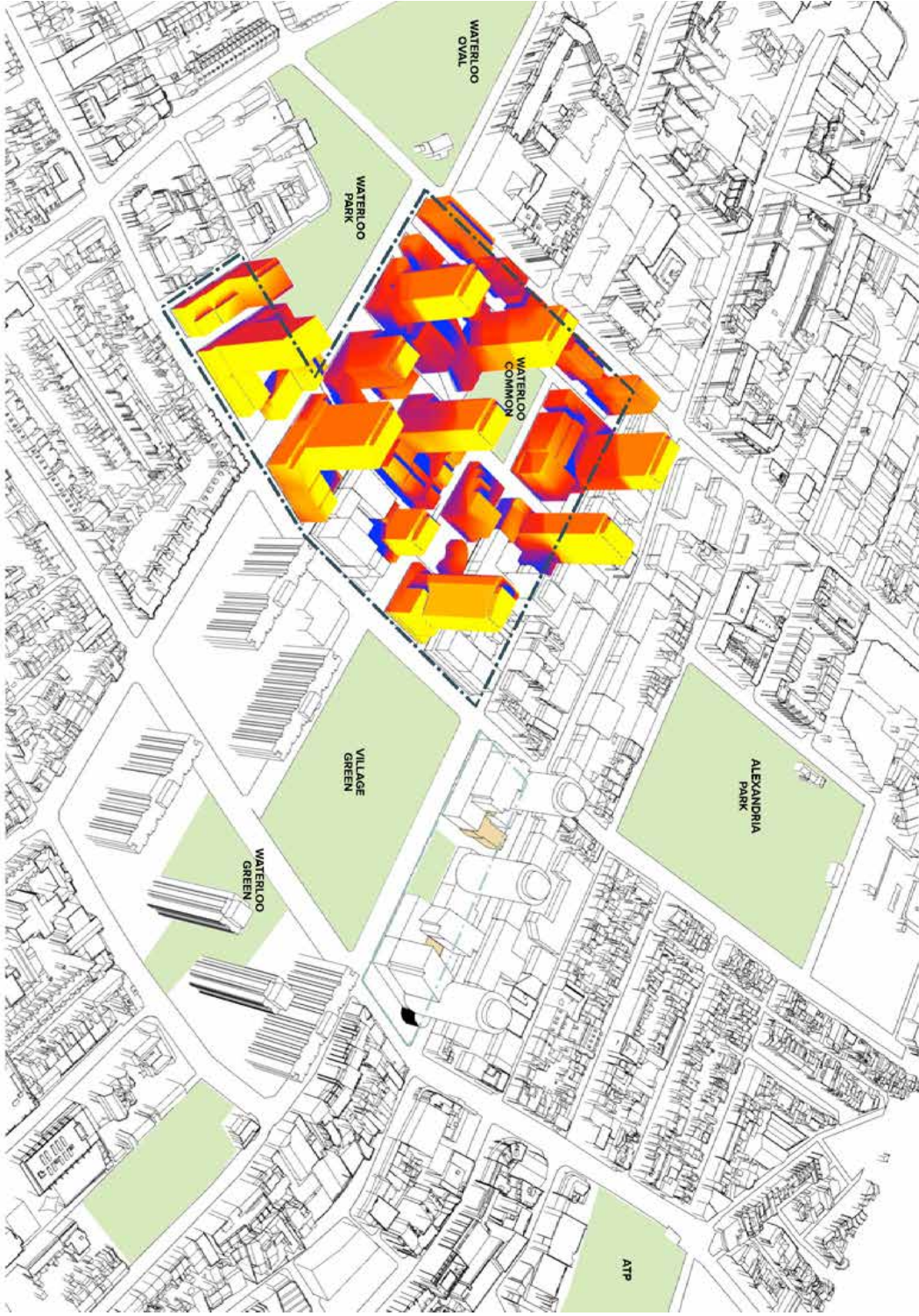
Fig. 7.9:98 Solar access to Waterloo South between 9am - 3pm mid winter, north east view
