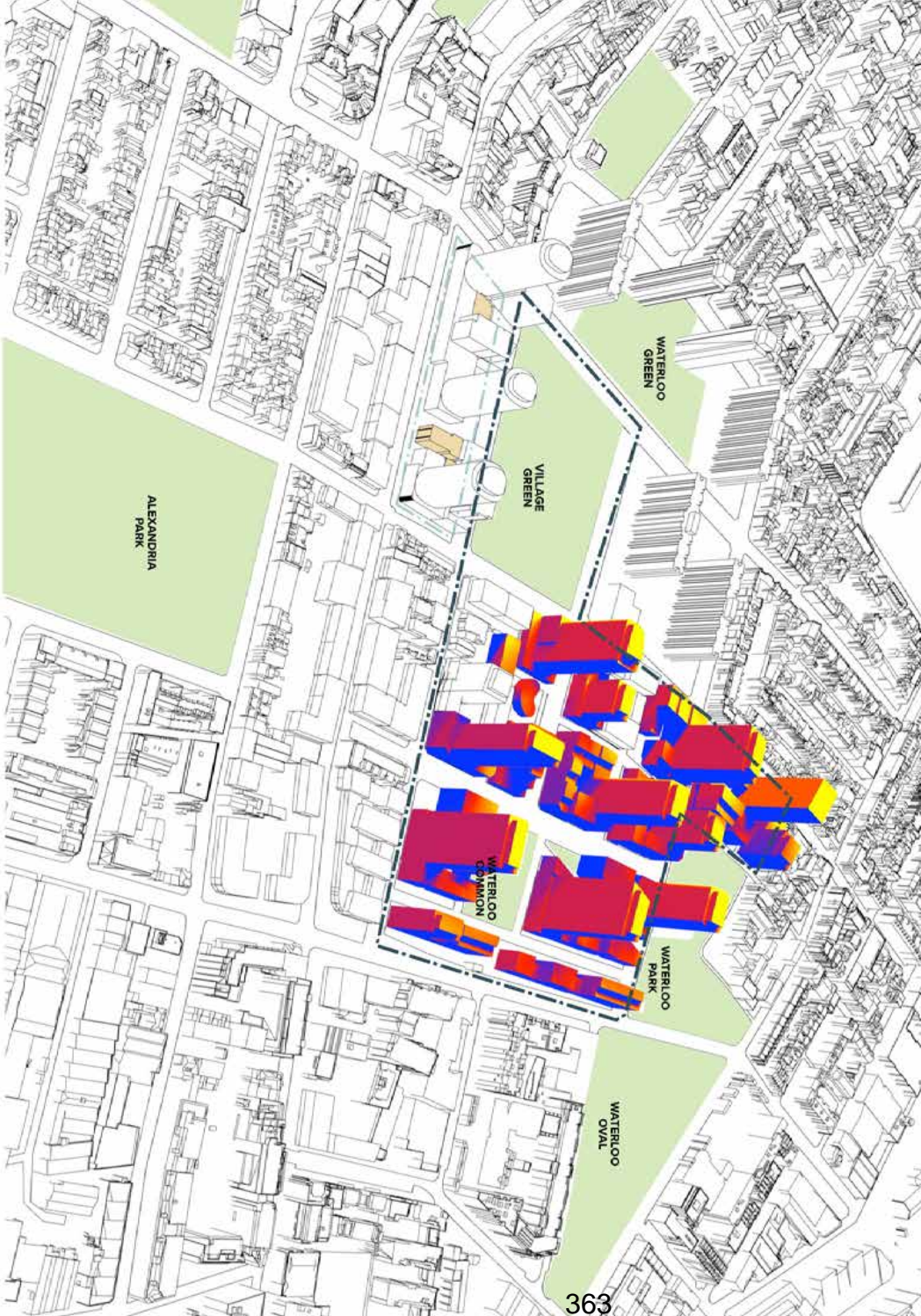
Fig. 7.9:97 Solar access to Waterloo South between 9am - 3pm mid winter, south west view
