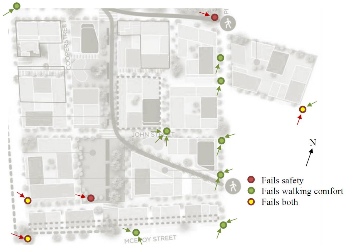
Figure 22 Wind impacts of LAHC's planning proposal request (see Appendix 26 to Attachment B)
