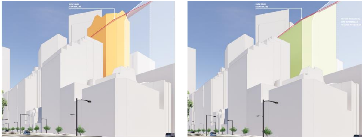
Figure 11 Existing sun access plane breach by the existing building (in yellow) and proposed envelope within the sun access plane (in blue)
