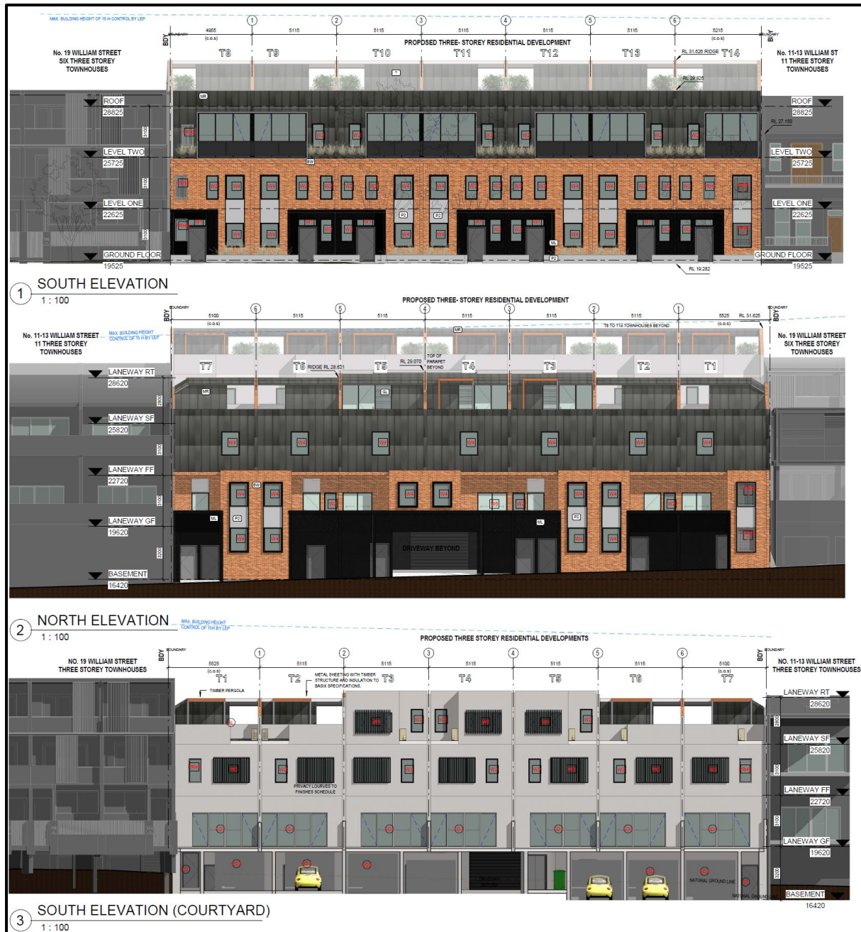
Figure 45: Extract of the North and South Elevations demonstrating that the upper levels are recessed from the levels below which reduces the perceived bulk of the proposed development
