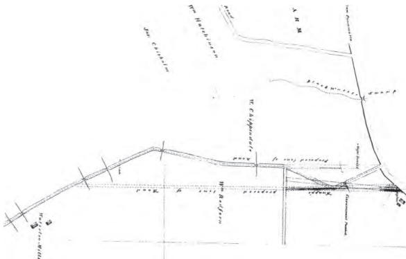
Figure 21: The alignment of Regent Street/Botany Road is shown in this plan of January 1842, prepared by Captain Wilson. The survey was undertaken to dedicate the road a parish road. Wilson recorded an existing alignment that was continued with, and another alignment following the future Botany (Cope) Street south to the Waterloo Mill recommended by Edward Knapp.
