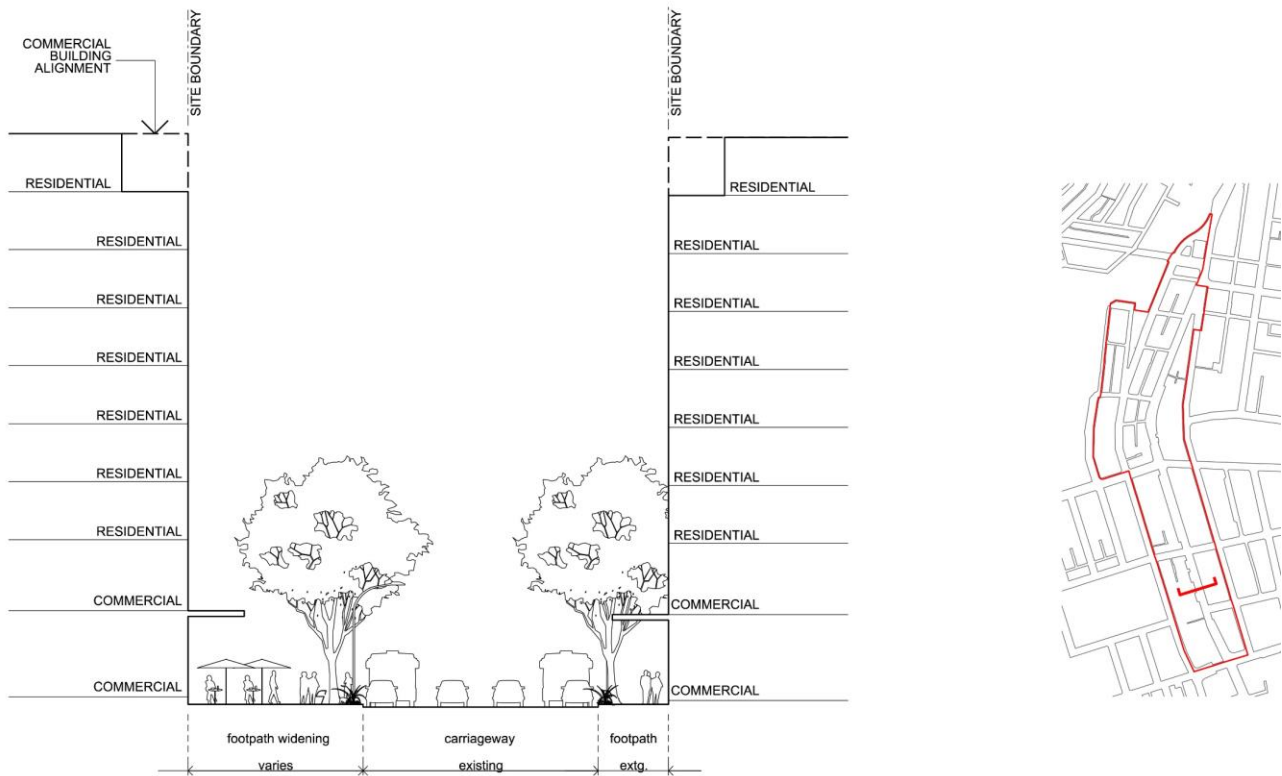
Figure 19. Street cross section through Botany Road between Wellington and John Streets looking north. Refer key map at right for location. Deeper building alignment setbacks along western side allow for greater pedestrian amenity, outdoor dining, tree zones and street furniture zones.
