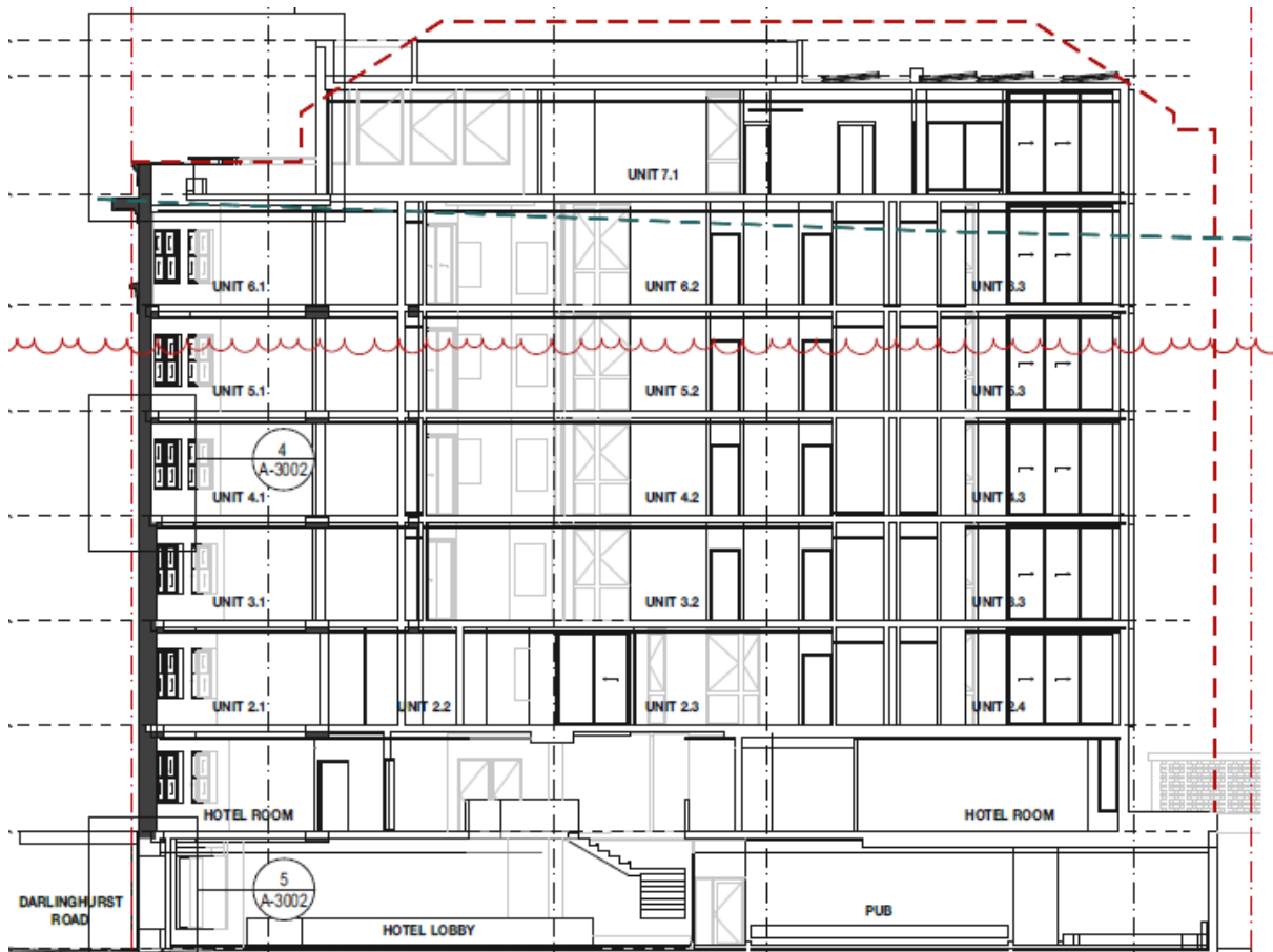
Figure 29: A section of the Commodore showing the areas of non-compliance above the 22m control
