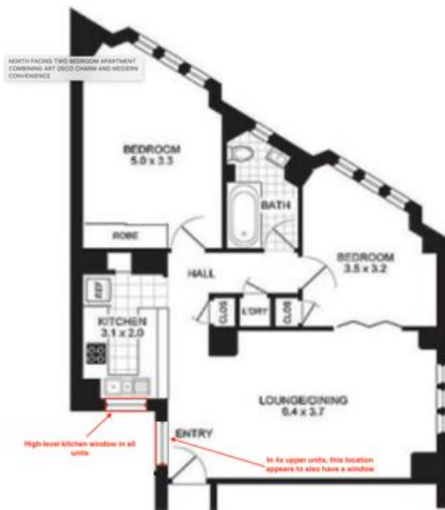
Figure 36: A typical floor plan of a unit layout at the front of Kingsley Hall, and adjacent to the lightwell
