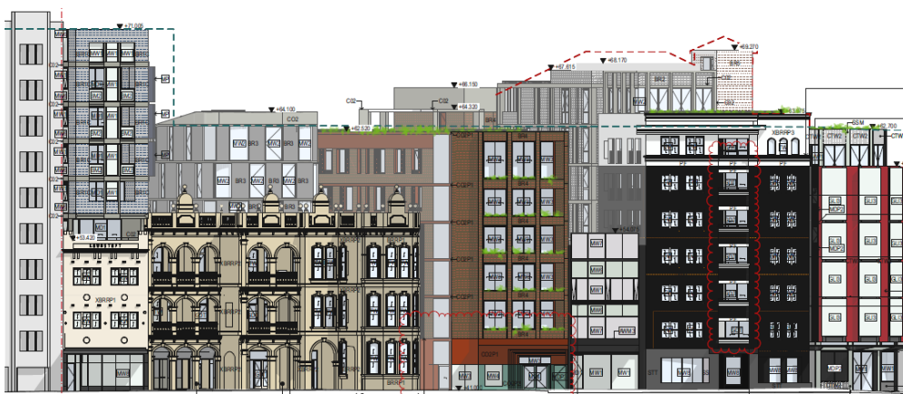
Figure 34: The proposed Darlinghurst Road elevation demonstrating compliance with the urban grain controls.
