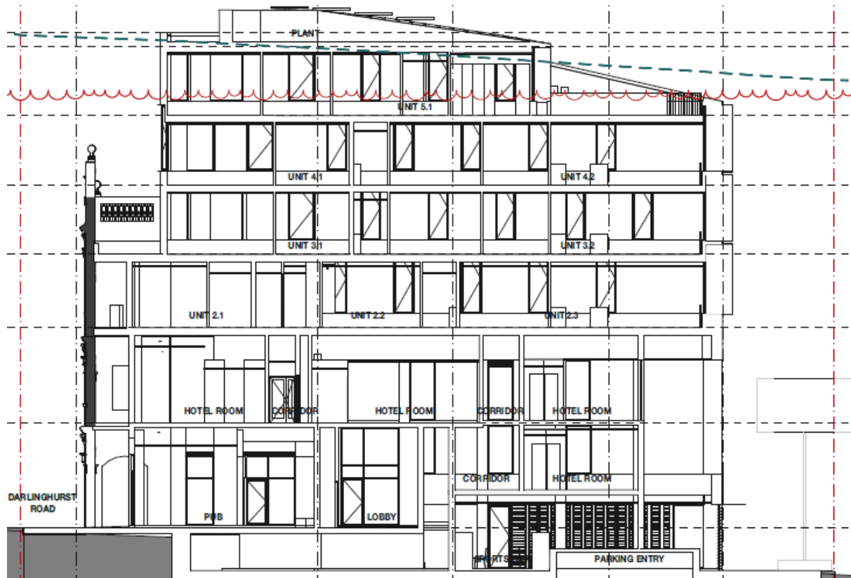
Figure 27: A section of the Bourbon showing the areas of non-compliance above the 22m control
