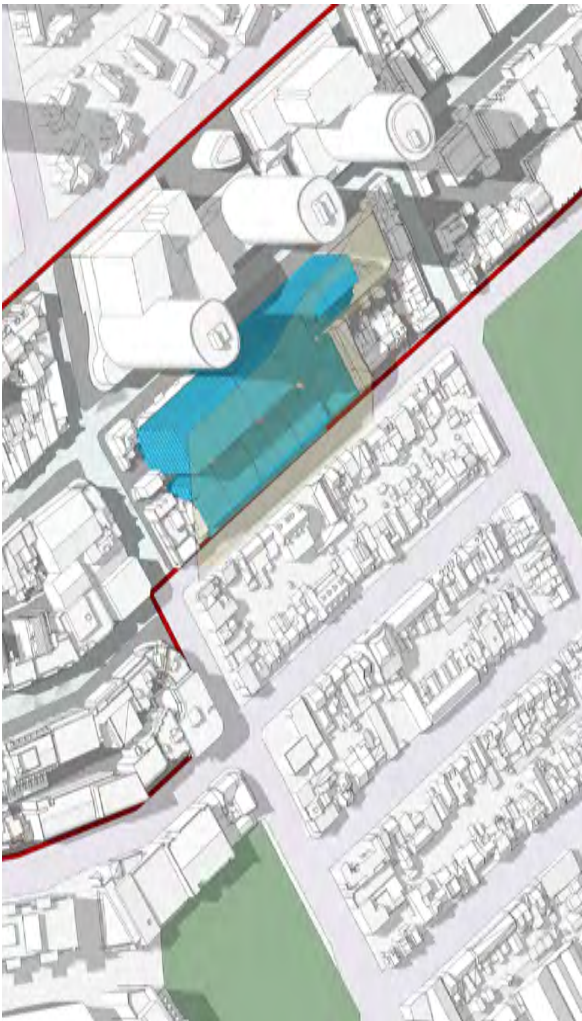
Figure 279: Waterloo Metro Quarter Precinct - proposed sun access plane to maintain solar access between 1030am and 1230pm (minimum 2 hours).
