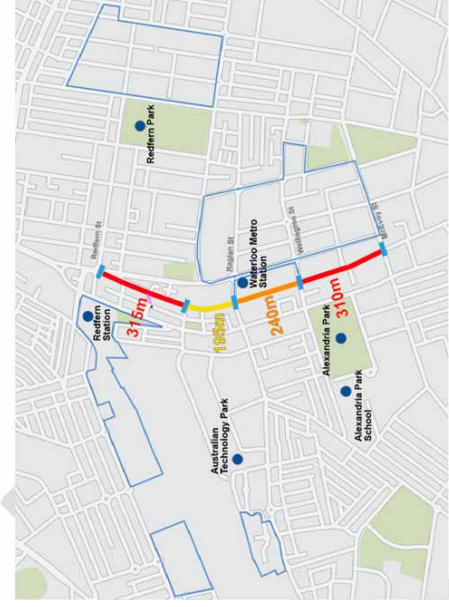
Figure 24: Existing distances between Botany Road pedestrian crossings
