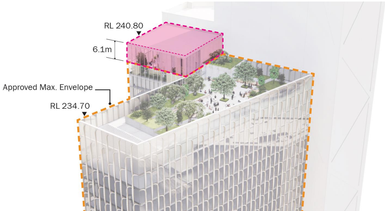
Figure 1 Three-dimensional view of the extent of variation to the approved 232 metres height plane
