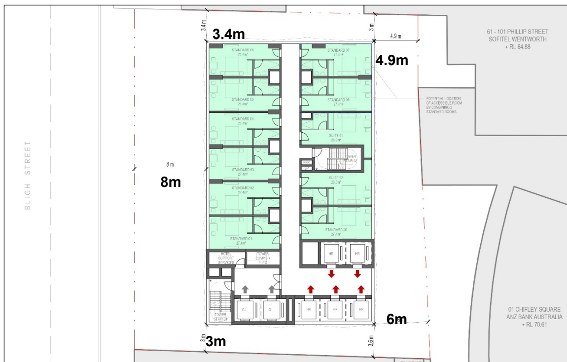
Figure 4: Indicative tower floor plate with setbacks shown
