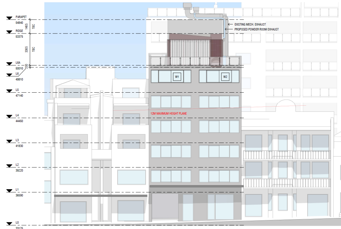
Figure 1: Extract from architectural plans prepared by Anton Kouzmin Architecture indicating breach of the maximum height control
