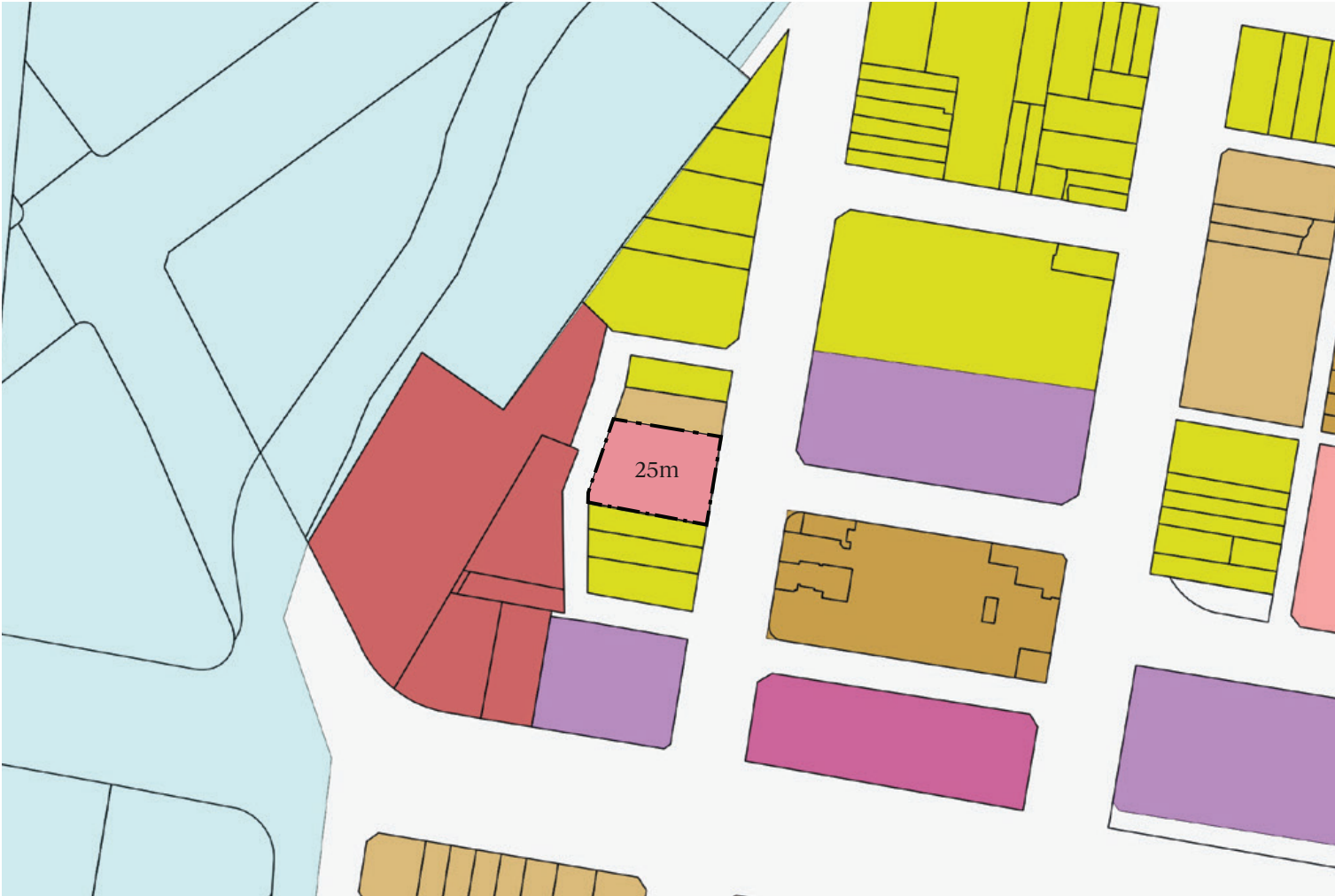
Proposed Height of Buildings Map (HOB) An increase in the permissible Height of Buildings for the site to 25m.
