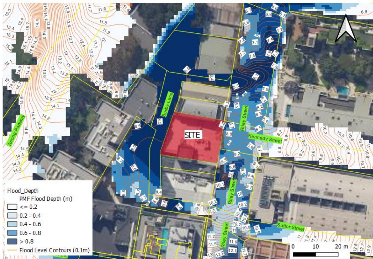
Figure 4. PMF Flood Extent (Flood Levels obtained from Council, Flood depths calculated from supplied DTM)
