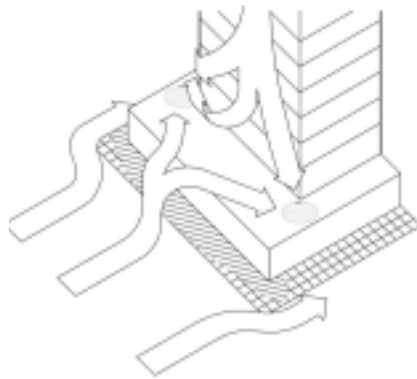
Figure 7: The tower-on-podium massing often results in reasonable conditions at ground level, but the podium may not be useable.
