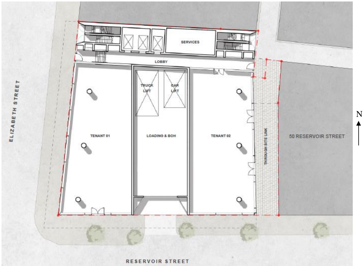
Figure 3: Ground floor of the proposed development.
