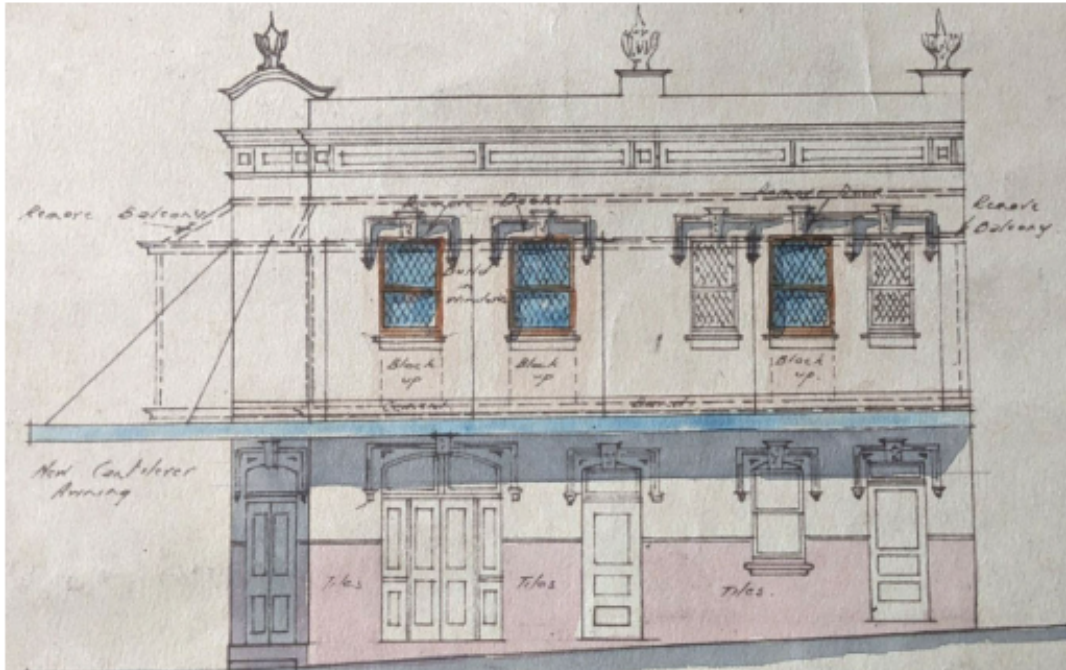
③ This elevation plan shows the Devonshire Street façade of the Clarendon Hotel with an outline of the original balcony to be demolished and a new awning. The 'Proposed alterations to Clarendon Hotel...for M Halpin Esq.' by architect Francis P Ryan, were approved October 1924. (City of Sydney Archives, A-00556071)
